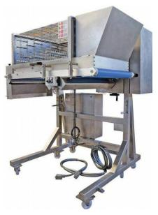
The dosing tape allows to garnish the food, sprinkling on its surface the grained product, with the intensity and quantity desired.
